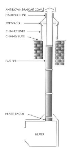
Installations shown complies with AS/NZS2918:2001. If a chimney exits out of the roof within 3 metres of the ridge the height shall be no less than 600mm above that point. If the Chimney exits further than 3 metres out of the ridge then it should project 1000mm above roof penetration. No part of the building may be in or above a circular area of horizontal radius of 3 metres from the flue exit.
