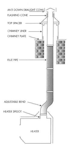
For optimum performance overall flue length should be between 4.2m and 4.8m and have no bends. Flue pipes should be 150mm in diameter. Due to factors such as roof pitch, predominant winds, nearby obstructions (i.e. trees, buildings), and fire placement, flue lengths, hats and cowls may vary.
