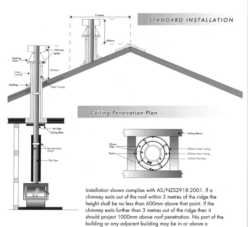
For optimum performance overall flue length should be between 4.2m and 4.8m and have no bends. Flue pipes should be 150mm in diameter. Due to factors such as roof pitch, predominant winds, nearby obstructions (i.e. trees, buildings), and fire placement, flue lengths, hats and cowls may vary.
