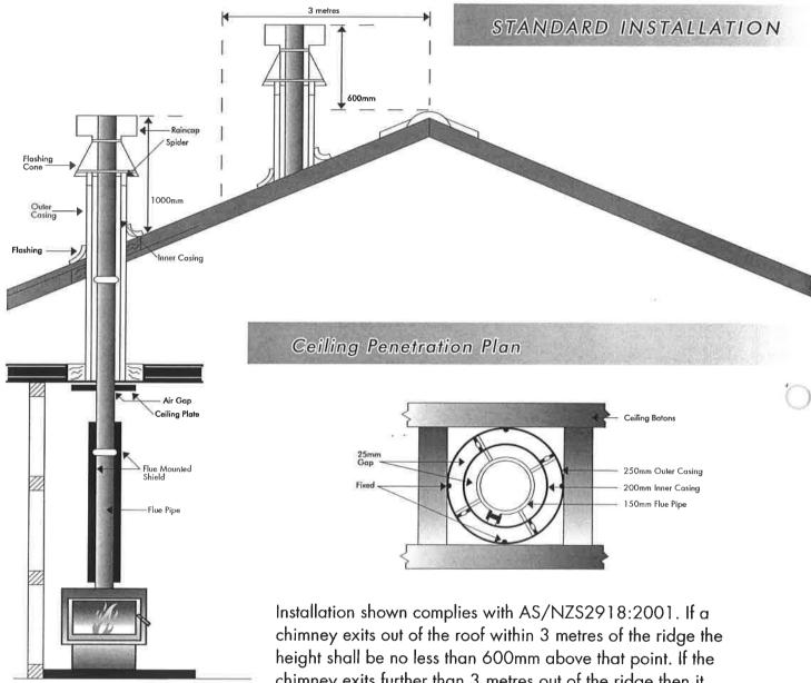
chimney exits further than 3 metres out of the ridge then it should project 1000mm above roof penetration. No part of the building or any adjacent building may be in or above a circular area of horizontal radius of 3 metres from the flue exit.
