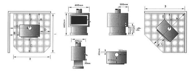
Minimum Clearance to Combustibles in Millimetres AS/NZS2918: 2001
