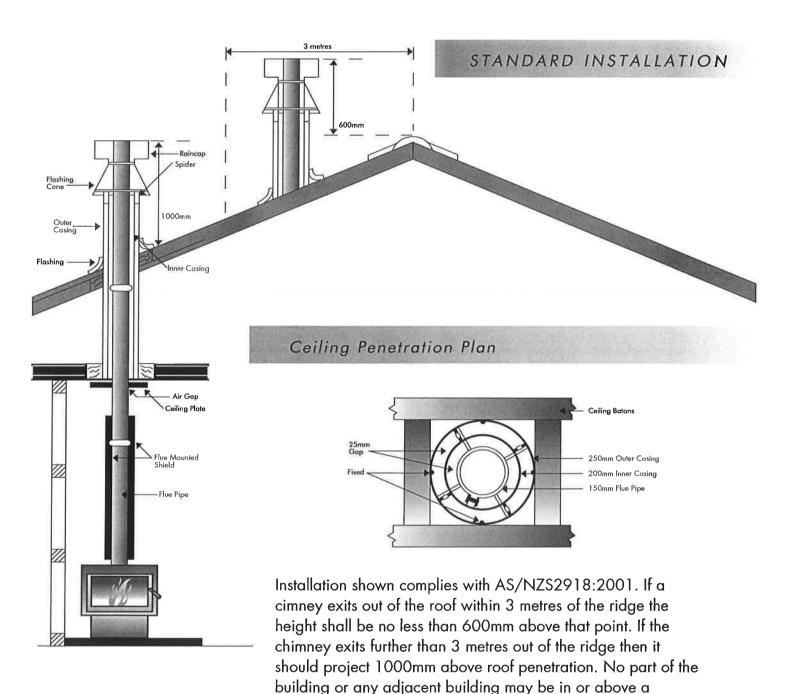
For optimum performance overall flue length should be between 4.2m and 4.8m and have no bends. Flue pipes should be 150mm in diameter. Due to factors such as roof pitch, predominant winds, nearby obstructions (i.e. trees, buildings), and fire placement, flue lengths, hats and cowls may vary.
