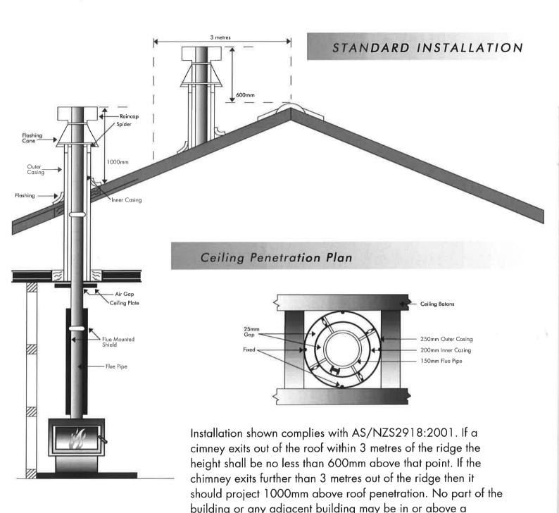
circular area of horizontal radius of 3 metres from the flue exit.
